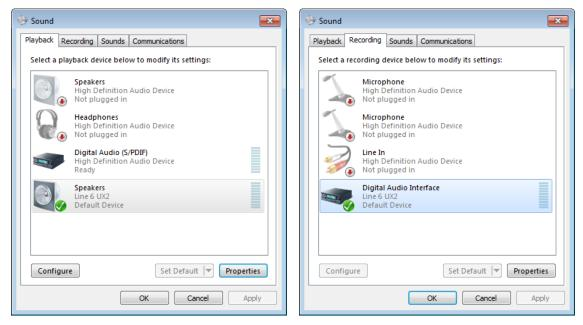
Select your Line 6 audio device in the Playback tab and choose "Set Default" if you want your applications to use it for audio playback. Repeat the same within the Recording tab to allow Windows® applications to use the device for recording as well.
