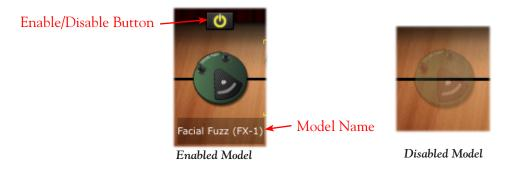
TIP: When a Guitar or Bass amp model is disabled, its Cab and Mic model remain active. This allows you to still have the speaker and mic emulation added to your signal. The Cab and Mic models can be independently enabled/disabled in the Cab View panel.
