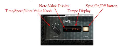
Please see the POD Farm 2 Plug-in **FX Time/Speed Control** descriptions on <u>page 3•11</u> for details. Functionality is the same for these Elements Delay & Mod Farm controls.
