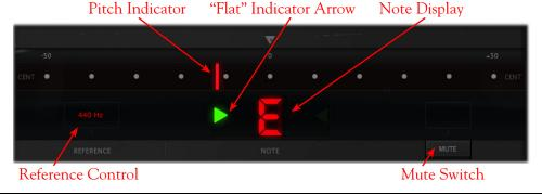
Note that you'll typically need to activate your DAW software's track "Input Monitoring" feature to feed your instrument input through the inserted POD Farm 2 Plug-In to allow the Tuner to receive the signal.
