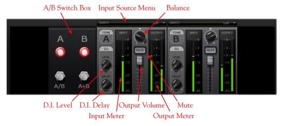
Input Source Menus - Depending on your DAW host software's features,\* when using the stereo POD Farm 2 Plug-In, you can select the input source (left channel, right channel, both channels) of the track's audio that is fed into each of the Plug-In's Tone Paths. (When using the Mono-Stereo version of Plug-In available in some DAWs, these Input Menus are not displayed.) Note that you'll see different options if POD Farm 2 Plug-In is running a Single Tone or Dual Tone configuration:
