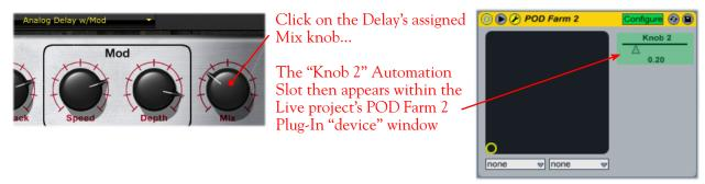
Configuring an "assigned" POD Farm 2 Plug-In parameter in Ableton Live
