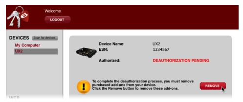
Line 6 devices that include Factory Add-Ons require the "Remove" step when deauthorizing
